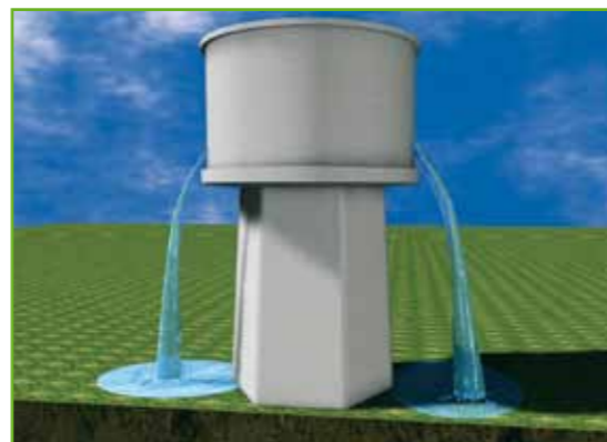
Filled water tanks cannot be accessed from the inside to apply a waterproofing layer. For an uninterrupted usage, waterproofing from the outside (negative side) is necessary.
