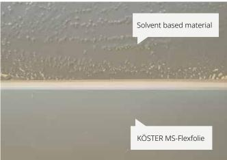
// KÖSTER MS-Flexfolie vs solvent based material applied on the same moisture content substrate
