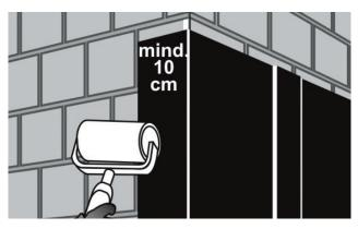
Apply the membrane on corners to the substrate on both sides of the corner by at least 10 cm.
