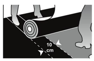
When applying the membrane overlap individual sheets by at least 10 cm.
