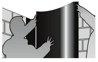
Overlap the KÖSTER KSK Membrane by at least 10 cm onto the piece of membrane applied in the corner.
