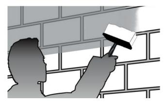
The surfaces have to be coated with KÖSTER KBE Liquid Film, diluted 1:1 with water using the KÖSTER Brush for Liquids. Mixture: 200 g/m<sup>2</sup> KÖSTER KBE Liquid Film plus water. Alternatively, the KÖSTER Primer BL with 150 g/m<sup>2</sup> can be used undiluted. In case of absorbent substrates the consumption can be higher.
