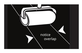
Sheets of membrane are placed so that the edges on longitudinal and transverse seams overlap by approx. 8 cm and at connections 10 cm. Use a roller to firmly press the membranes onto the substrate. On overlapping areas, take special care to ensure that the membranes have been pressed together well. When used for sealing in and under walls, the overlap must be at least 20 cm. The waterproofing according to DIN 18 534 is carried out in one layer up to water exposure class W2-I.
