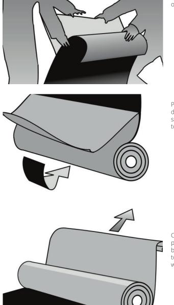
Pull the backing paper off on a length of 20 cm.
