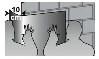
Remove the backing paper on a length of approx. 20 cm, align the KÖSTER KSK Membrane and apply it to the substrate. KØSTER
