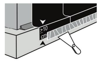
Seal the lower edge with KÖSTER KBE Liquid Film.
