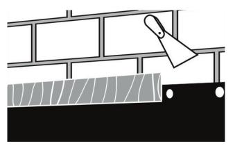
After fastening, the upper seam must be secured against leaking from behind. To do this, the area should be filled with KÖSTER KBE Liquid Film.
