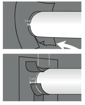
Cut a hole with the diameter 2 cm smaller than the pipe into a piece of the KÖSTER KSK Membrane and bond it to the substrate, ensuring that no air is enclosed under the membrane. If the pipe penetrations are already connected, cut the blank on the side and pull it around the penetration. Always glue the edge of the cut to the opening by at least 1 cm.
