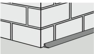
Round out edges. Install fillets in the wall / floor junction using KÖSTER WP Mortar. Close voids and holes using KÖSTER WP Mortar.
