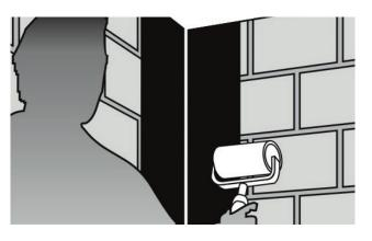
On inside corners, apply a piece of membrane at least 30 cm wide into the corner area.
