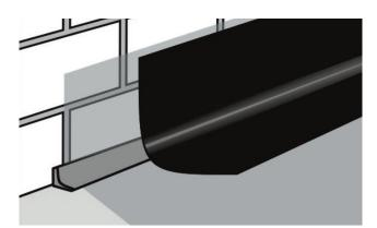
After the fillet has been installed, reinforce the wall/floor junction by applying an at least 30 cm wide stripe of membrane over the fillet. The cut should reach approx. the upper edge of the screed.
